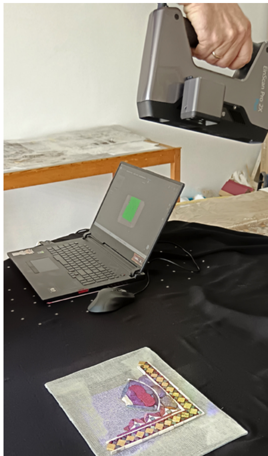
3D scanning of the reverse side of the corner decorative unit with floral ornament (photo Mishko Tutkovski)
