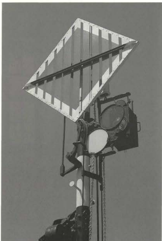
Signalling mechanism: "The signalman moved a switch to its left or right position by moving a certain lever, thus opening or closing the signal." .....
