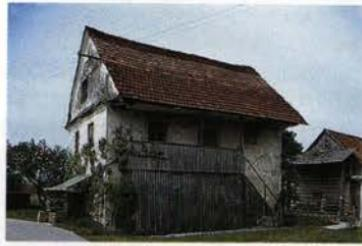
The roof is of a symmetrical pitched type. The ridge terminates in two hipped ends. The roofing consists of tiles.
