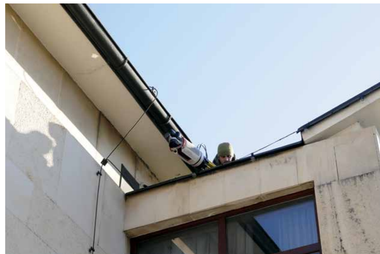
4. Stojišče inštrumenta tik ob steni objekta za skeniranje zadnjih površin ter postavitve inštrumenta na strehi za skeniranje zgornjih površin doprskih kipov (foto: Jon Grobovšek, 2012) 4. Scan location of the instrument right next to the wall of the building to scan the rear surfaces and positioning of the instrument on the roof to scan the upper surfaces of the busts (photo: Jon Grobovšek, 2012)
