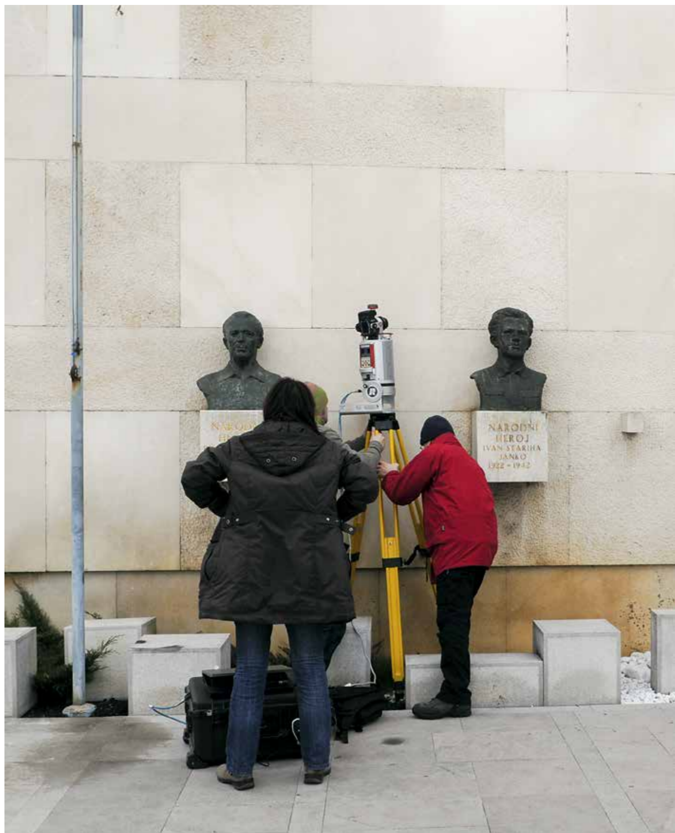
3. Terestrični laserski skener s fotoaparatom na stojšču (foto: Jon Grobovšek, 2012) 3. Terrestrial laser scanner with camera in scan location (photo: Jon Grobovšek, 2012)
