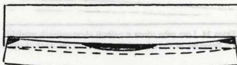
Skica 21. Cone naleganja utorne letve v utoru kot posledica krivljenja table (označene s temno barvo) Fig. 21 – Zones of the subsiding of the groove small board in the groove as a consequence of the bending of the board (marked with dark colour)
