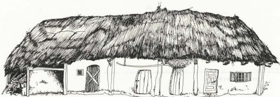
Sl. 1 Dubrovnik šte. 127: stegnjen dom, lesena ometana hiša z ločenimi vhodi v posamezne prostore z dvoriščne strani (risal I. Cerkvjenik) Fig. 1 Dubrovnik No. 217: a stretched house, a wooden plastered house with separate entrances to the individual rooms from the back-yard side (Drawn by I. Cerkvjenik)
