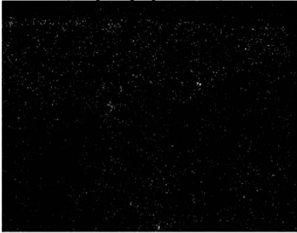
Figure 9: Distribution of sulphur by EDS mapping analysis in the sample after 1 hour of application of ammonium carbonate in carbogel. ( w_S = 0,28\% )
