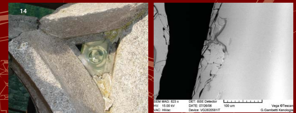
14. A piece of original window glass (left) and SEM image of the glass cross-section (right) from the Gothic period
